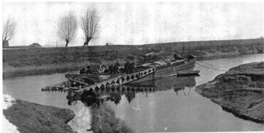
WIDDOP-ENGINED "BRODER," A SPECIAL TYPE OF DREDGING CRAFT BUILT FOR THE OUSE DRAINAGE BOARD FOR KEEPING CLEAR THE RIVER FAIRWAYS.
